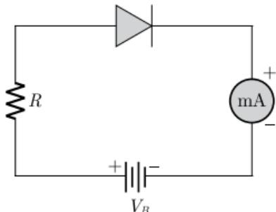
29.I. If  $V_B = 5$  V, the value of R in order to establish a current to 6 mA in the circuit is [ 1 ]
