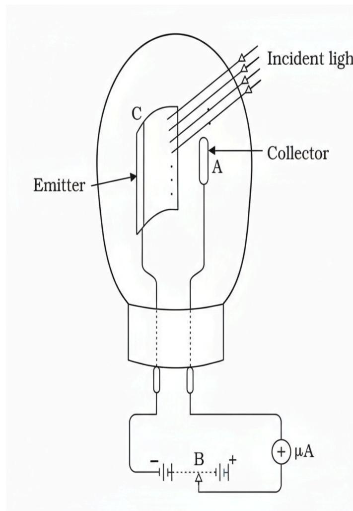
30.I. If a retarding potential is applied by moving the terminal B towards the left, how will it affect the [ 1 ] microammeter reading?
